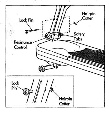
To use the upper body arms in the dual motion position, first make sure the resistance control is tightened. Remove the lock pin from the upper body arms and the upright, and insert it through the safety tabs at the base of the upright. Insert the hairpin cotter into the lock pin.
